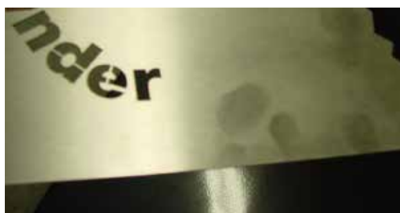
Fig. 3.2.5 Fingerprints beneath clear coat
