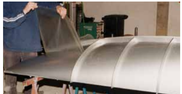
Fig. 5.2.4 No or poor inter-coat adhesion
