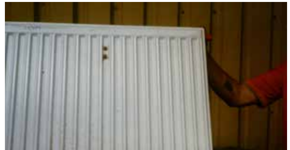
Fig. 5.2.2 Pretreatment unsuitable or insufficient
