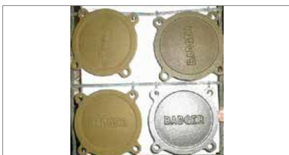
Fig. 1.3.6 Corrosion of sandblasted workpieces after pretreatment
